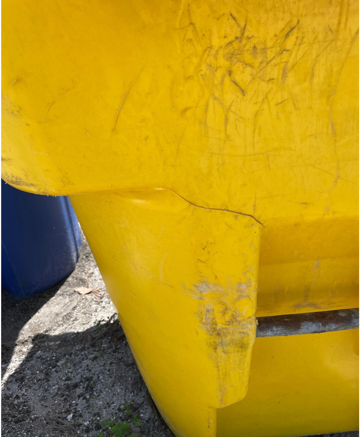
CAMDEN G- CRACKED YELLOW TOTE. REPORTED IN BY A CV UNIT OWNER. A REQUEST FOR REPLACEMENT WAS SENT TO WASTE PRO.
