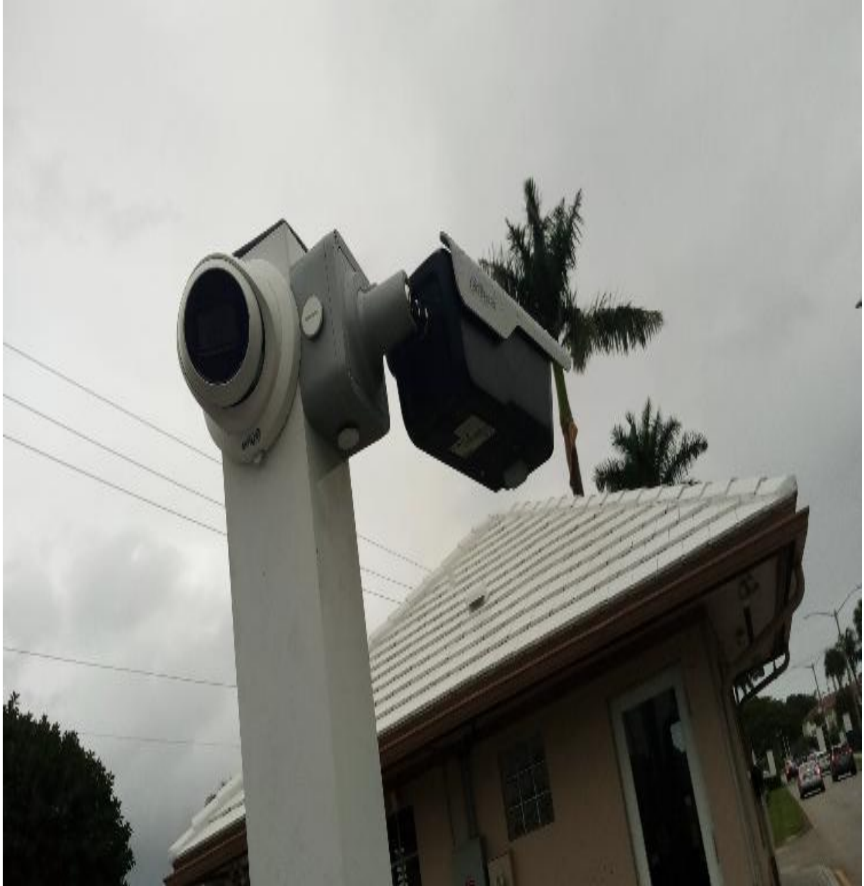
OKEECHOBEE BOULEVARD ENTRANCE- THE NEW CAMERA ON THE RIGHT CATCHES LICENSE PLATE INFO AND SENDS IT DIRECTLY TO THE GUARDHOUSE COMPUTER.
